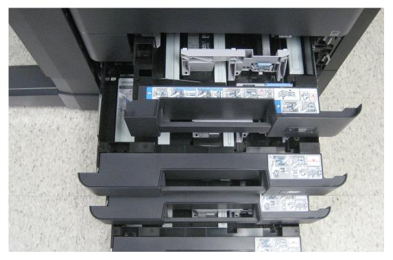
Both length and width guides slide in the drawers when adjusting paper size. In addition, stickers available on side to side guides are easy to read and break down different height limits from standard paper to envelope height. Plus, the soft close drawers make for no slamming of cassettes.
