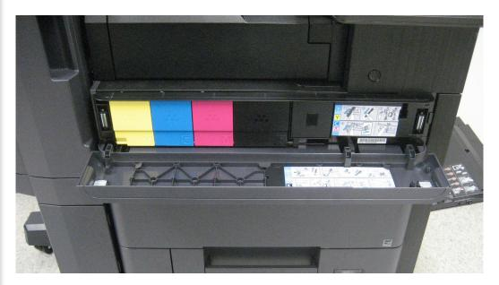
The process for replacing toner is simple and clean, and toner can be replaced on the fly. Further, an expired black toner bottle can be used as a waste toner container, reducing waste, as well as storage requirements for the customer. A Summer 2016 Outstanding Achievement in Innovation winner, making the change is a cinch, with users only needing to remove the toner bottle, flip it around, and insert it into the waste toner container compartment at the front of the device.
