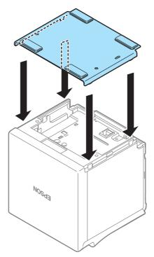
**2** Hook the catches into the bottom cover and attach the rear cover to the printer.
