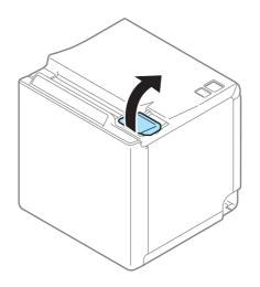
**2** Remove the used roll paper core if any, and insert the roll paper.
