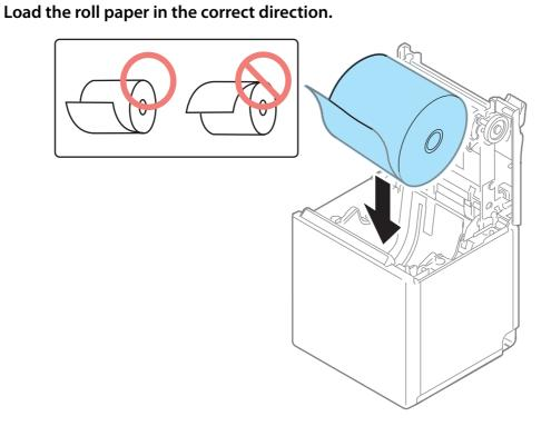
**4 Pull out some paper, and close the roll paper cover.** When the printer power is on, the roll paper is automatically cut.
