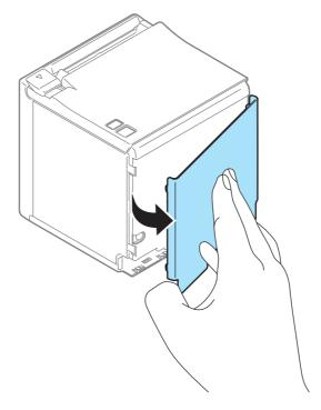
**2** Use your finger to remove the bottom cover as shown in the illustration.
