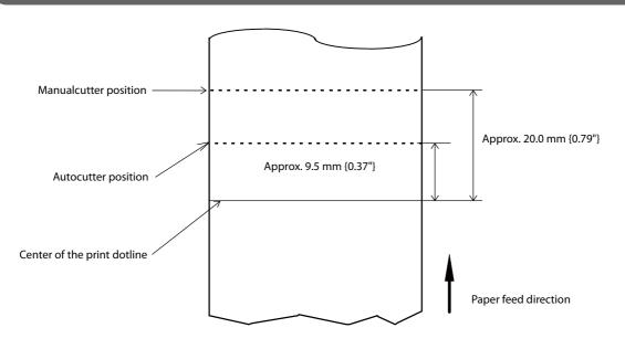
• The values above may vary slightly as a result of paper slack or variations in the paper. Take this into account when setting the cutting position of the autocutter.
