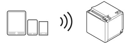
SimpleAP mode is enabled by default when shipping from the factory. When SimpleAP mode is enabled and the printer is turned on, the following information is printed automatically.
